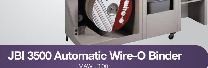
The JBI 3500 Binding Machine provides high-speed Wire-O finishing 'on-demand' from cost-efficient spools. At 500-1000 books per hour, the Wire-O Bind is superfast, yet simple to operate with all size and format setups instantly adjustable by user-friendly 'touch screen' electronic controls. This machine automatically cuts wire to length, feeds and positions wire for insertion; accurately sends book to patented closing station, and delivers book to standard pile reception unit.
